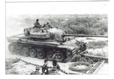
It detonated 73 mines [18%] of the 400, with 1/3<sup>rd</sup> believed to have been caused by the tank tracks, which caused excessive, unsatisfactory damage to the tracks and suspension stations. A brainstorming session with 1 Field Squadron Officers and NCOs created a number of new methods, of how to deal with the minefield destruction.
